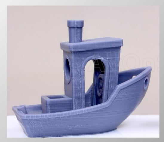
But, DLP the prints have very good surface detail and high resolution with small features possible.
